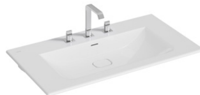
Rectangular vanity basin with overflow hole, 3TH, 100cm H: 172mm W: 995mm P: 530mm
