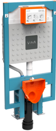
Regular wall-hung frame, 8cm, floor fixation with electrical connection, 3/6 litre
